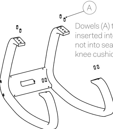
Dowels (A) to be inserted into the runners, not into seat or knee cushions.
